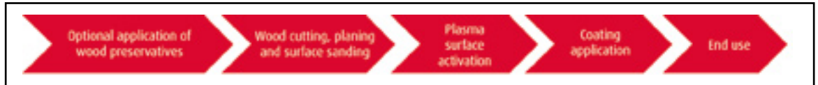
Figure 4: Stages in the "Durawood" plasma pretreatment of wood surfaces (preferably in-line with coating)
